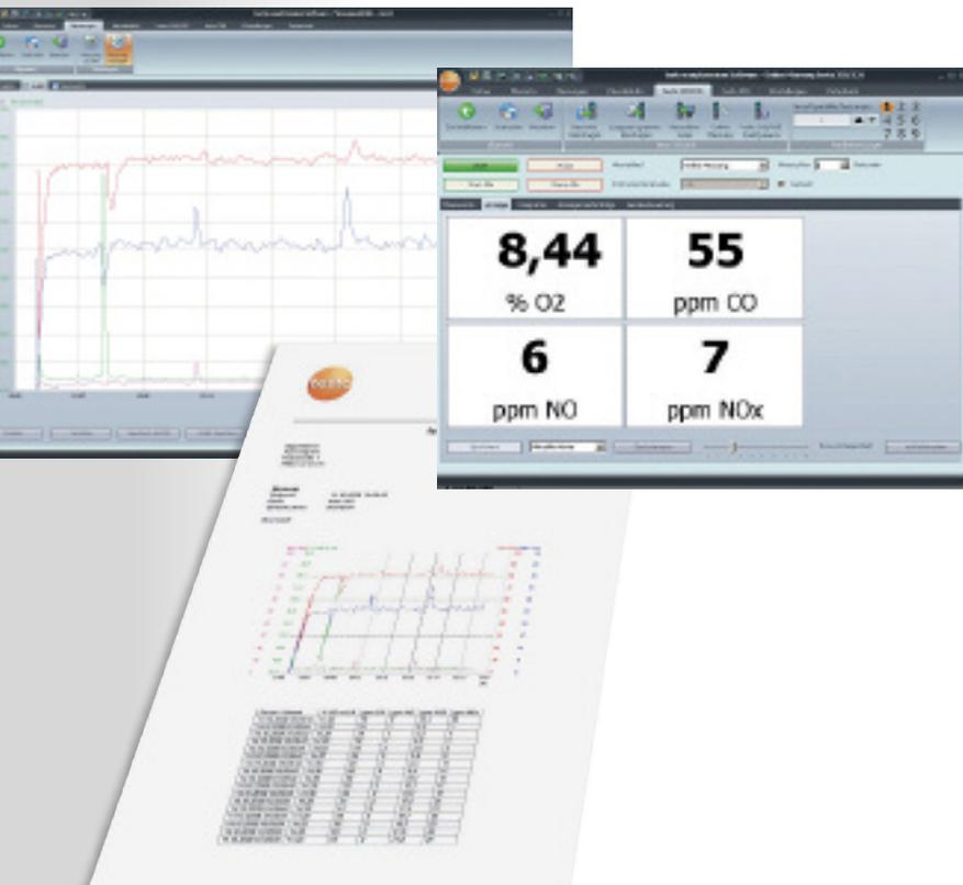
Data can be read out, easily edited, filed and managed using "easyEmission" software:
