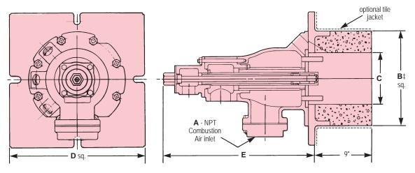
**NOTE:** For 6422-8-A, air and gas connections cannot be piped in the same plane because the "flower pot" type air connection flange would interfere with the 2½" gas line.
