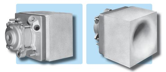
**4831 Flat Flame Burners** transfer heat to the surrounding refractory wall or roof by highly turbulent convection; the refractory then radiates heat uniformly to the load. Minimum forward velocity results in uniform radiant heating with no flame inpingement.
