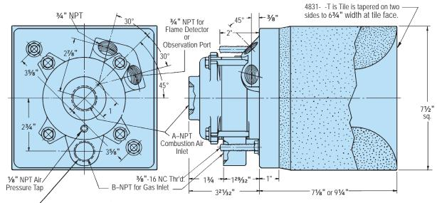
Z With pilot and flame detector bosses in position shown, gas inlet can be positioned at either 6 or 9 o'clock positions.
