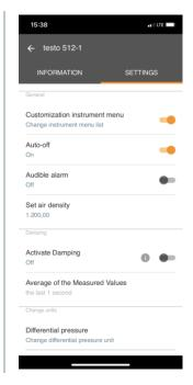
Changes to the measuring instrument settings in the app are transferred directly to the measuring instrument. Synchronization with the app is confirmed on the measuring instrument via "SYNC DONE".
