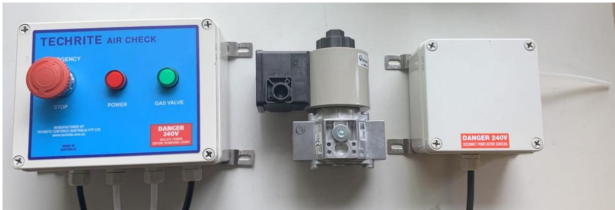
The Techrite Air Check is a self-contained device designed to prove the air flow in a ventilation system. Techrite Air Check consists of the Air check control panel (240 VAC), connected to an enclosed air pressure switch via 4 metres of cable. This can then be connected to any AS gas approved shut off solenoid valve (Single SSOV/Gas Valve) (240 V AC).
