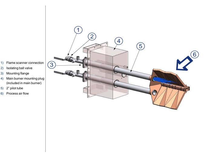
2 LVDT/HC-pilot burners mounted on a burner mounting plug, firing into a MAXON AIRFLO® "HC" line burner (burner mounting plugs standard available from MAXON on AIRFLO<sup>®</sup> "HC" and DELTA-TE<sup>™</sup> burners).
