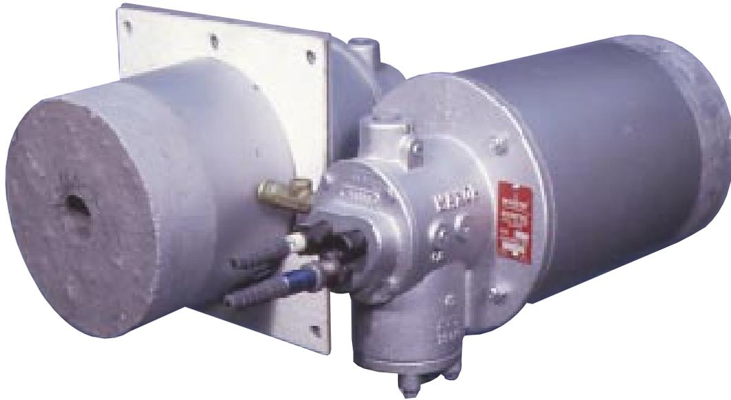
1-1/2" RAMFIRE® Burners: At right, burner assembly with UV scanner (supplied by customer), spark ignitor and optional mounting plate. Basic burner with standard refractory block and seal and support assembly is shown at left.
