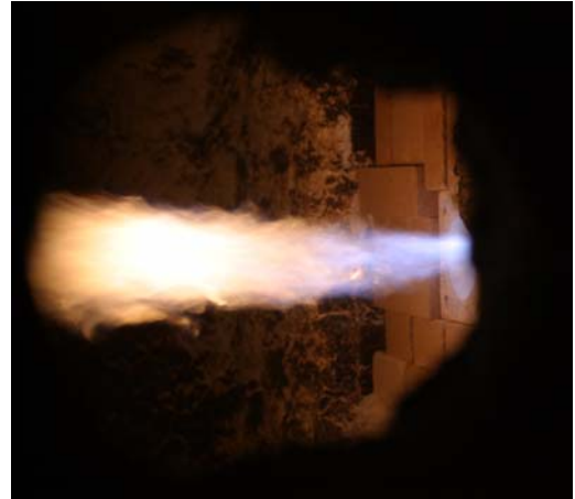
OXY-THERM® LE staged flame pattern
