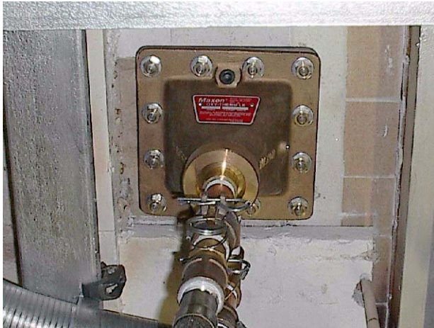
OXY-THERM® LE mounted on a glass furnace
