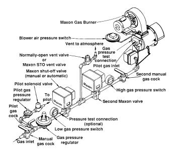
Model "400" OVENPAK<sup>®</sup> Burners provide the air supply (except for EB versions, which require a separate combustion air blower). They also serve as a fuel flow control and fuel/air mixing device.
