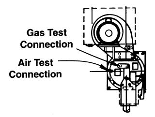
Determine your differential air pressure reading by taking an additional reading with manometer connected between the burner's air pressure test port and atmosphere with the burner at high fire position, fuel valves closed, and all air handling systems running. Subtract the combustion chamber static pressure obtained above from this air pressure reading to give you differential air pressure reading.
