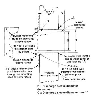
For pull-through systems, spacers may be installed on stud bolts and area D left empty to admit cooling air past the sleeve.
