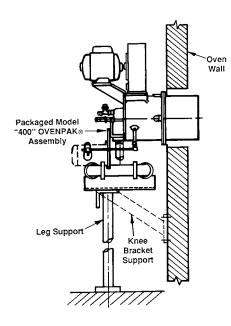
Additional burner support may be required in conjunction with a stiffener plate when mounting OVENPAK<sup>®</sup> Burner (weighing 100-350 pounds) through typical thin wall of heater/oven panels.
