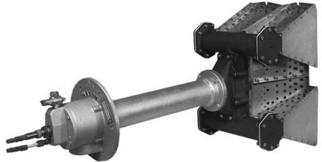
36" back inlet "H" INCINO-PAK® Burner section shown with (4) COMBUSTIFUME® Burner end plates; includes spark ignitor, pilot gas adjustable orifice cock, raw gas pilot, and arranged for mounting of customer's UV scanner
