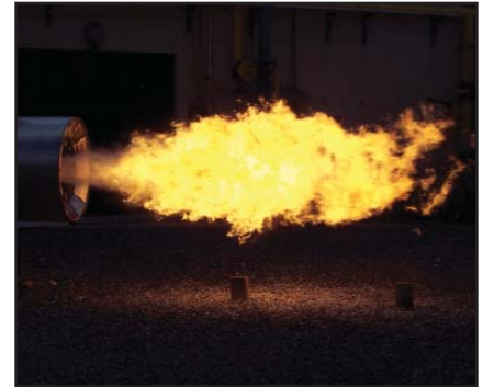
Eco-Star II 150 High Fire @ 160 MM Btu/hr (42,300 kW) - No. 2 Fuel Oil Low Pressure @ Low Spin Setting
