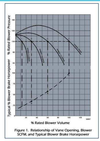
The control sequence is illustrated in the figure above. If the demand on the blower is decreased in volume from a normal operating point F, to another normal operating point G, the vanes close to a new position providing the new flow and maintaining the pressure equal to that at point F.
