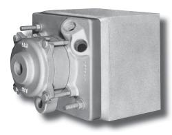
**4831 Flat Flame Burners** transfer heat to the surrounding refractory wall or roof by highly turbulent convection; the refractory then radiates heat uniformly to the load. Minimum forward velocity results in uniform radiant heating with no flame inpingement.
