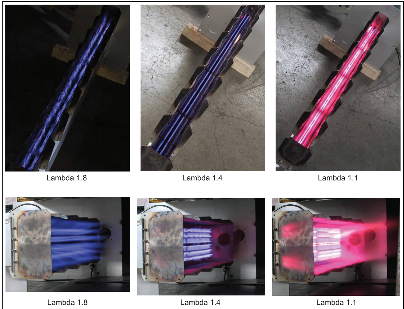
Figure 4.1. Low Fire Flame Appearance
