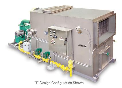
recirculation fan, combustion chamber, burner, combustion air blower, gas train and control panel mounted on a painted carbon steel skid. Ingress Protection ratings are available to suit all environments. The gas train and burner safety system are NFPA 86 or EN 746-2 compliant. The heater unit is built with high quality 304 stainless steel.
